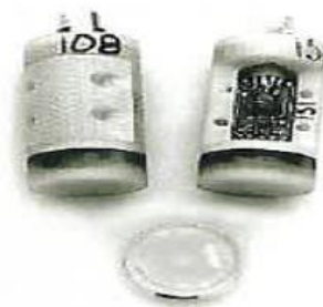
Figure 8: A HTS SQUID device from Tristan Technologies which contains a chip with a superconducting ring. The ring has one or more Josephson junctions. When a current, larger than the critical current of Josephson Junctions is introduced into the SQUID a voltage appears that is proportional to the magnetic flux through the SQUID ring. It can measure magnetic fields down to 10^{-14} [48]. Figure courtesy of T.M. Silver, S.X. Dou and J.X. fin, Institute for Superconducting and Electronic Materials, University of Wollongong, Wollongong, NSW2522, Australia .
