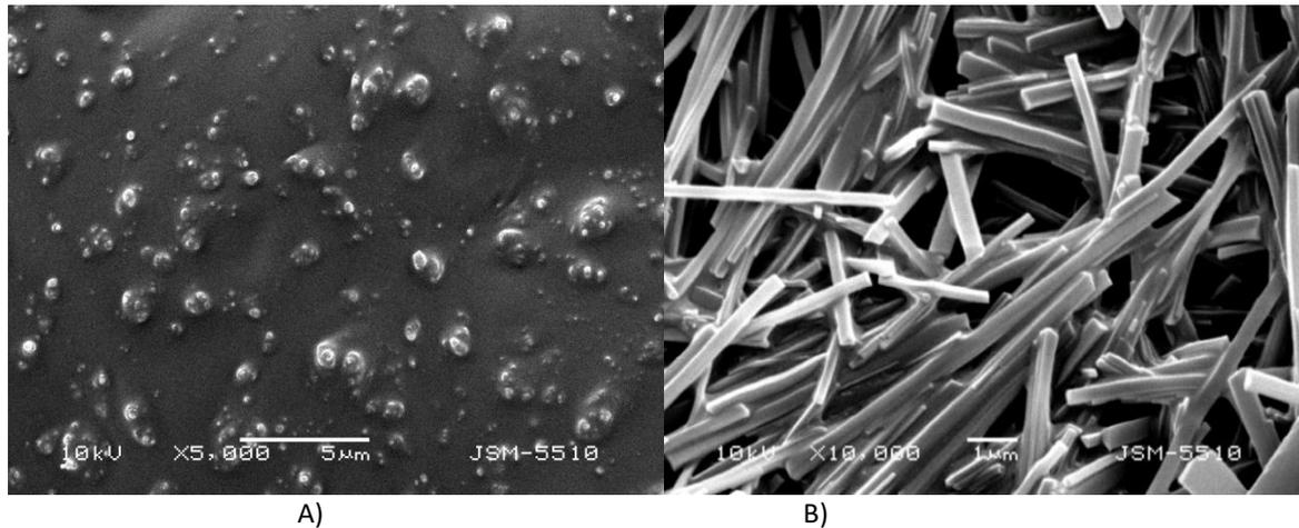
**Fig 4: Biofilm formed by *L. fermentum* Ts on the surface of mild steel, visualized using SEM. (A) Steel plates after corrosion in seawater with inhibitor supernatant obtained of mixed 10% maltose; (B) control—steel plates after corrosion in HCl.**
