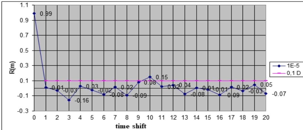
**Figure 3: Normalized autocorrelation function of the absolute error of the input samples**
