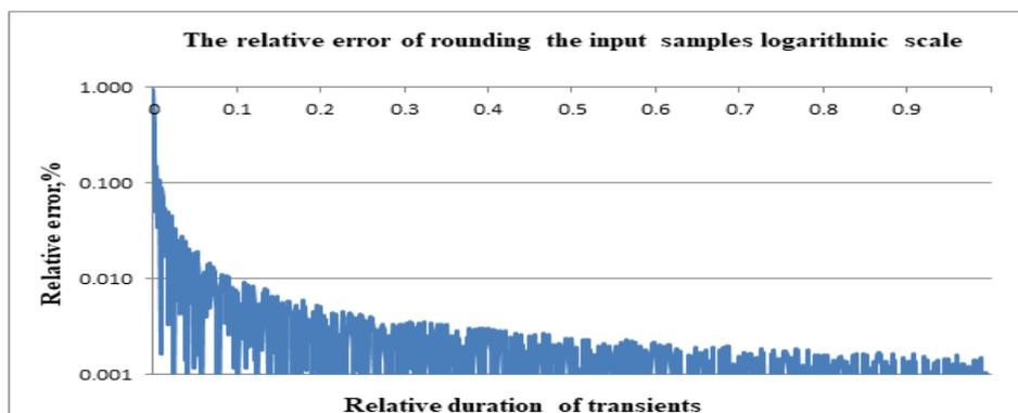
Figure 2: The change in relative error depending on the duration of the transition process
