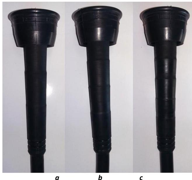
**Figure 1: General view of the teat tubes of the milking machine with the number of steps : a) - three; b) - four; c) – five**
