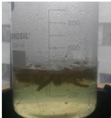
**Figure 3: Extraction of bagasse under boiling condition,**
