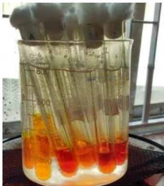
**Figure 8: DNS method of reducing sugar estimation of samples,**
