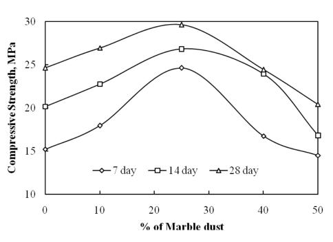
Figure 4: Influence of marble dust in compressive strength of mortar cube
