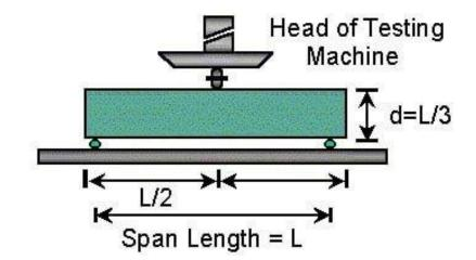
Figure 5: Schematic representation of flexural testing
