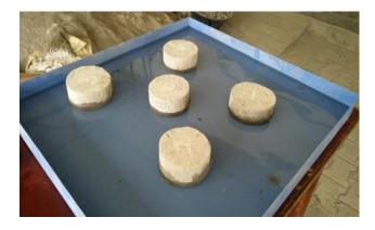
Figure 8: Mortar cube with marble power under water absorption
