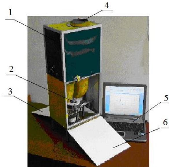
1-body, 2-actuator, 3-guide for untreated ears, 4-loading window, 5-control unit, 6-guide for cleaned ears
