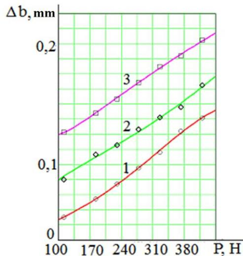
1 - area of the sheet start; 2 - zone of the middle of the sheet; 3 - zone end of sheet
