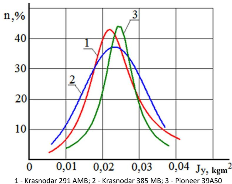
**Figure 9: Density of distribution of moments of inertia relative to the longitudinal axis of the cob**
