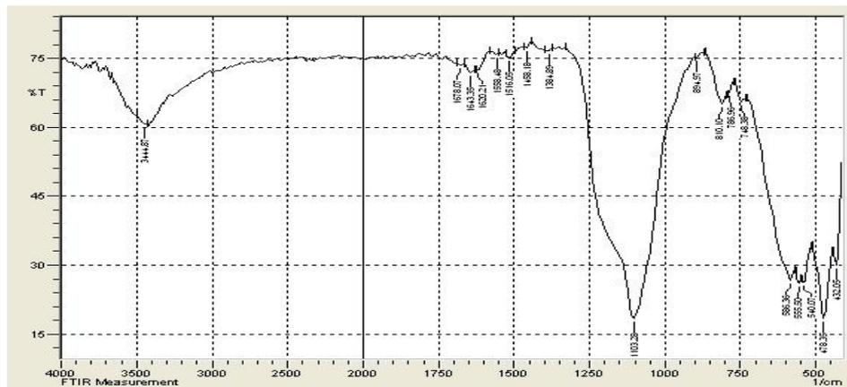
**Figure 1: FTIR for zirconium silicate nanofiller**
