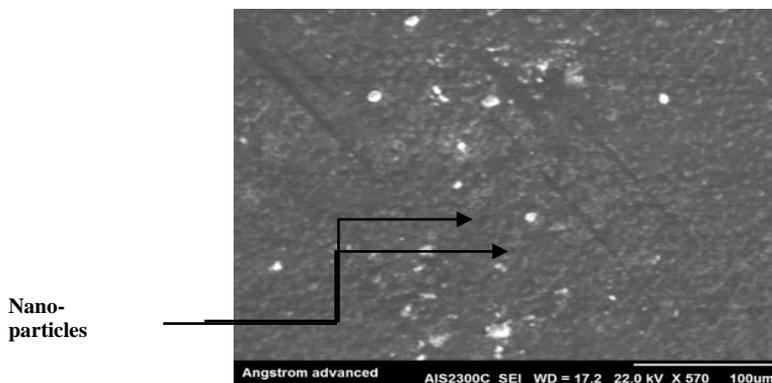
Figure 5: Scanning electron microscope of silicone/nano-composite with 100um magnification showed dispersion of nanoparticles
