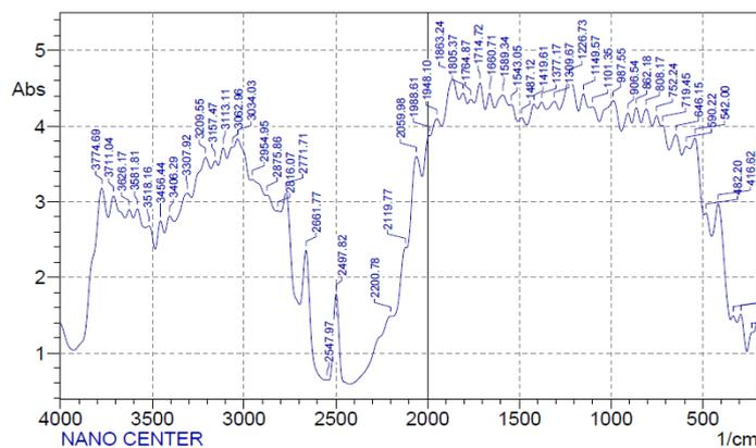
**Figure 2: FTIR for control sample of silicone.**
