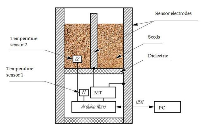
Figure 1: General view of the USB moisture meter
