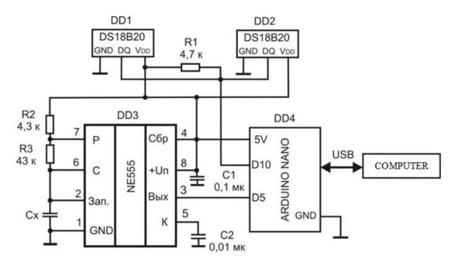
Figure 2: Schematic diagram of the USB moisture meter
