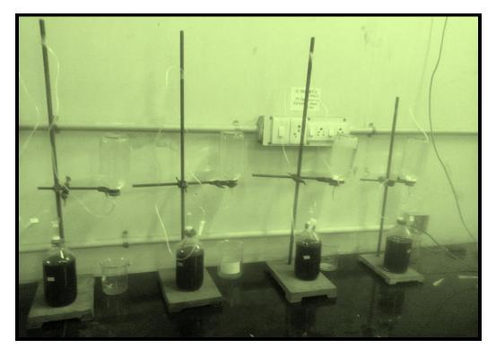
Figure 1: Experimental Setup for Biogas Production
