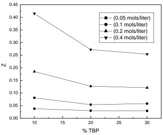
Figure 3:Loading ratios for the extracion of Acylic acid using modified oil
