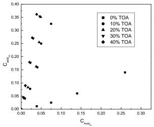
Figure 5: Chemical equilibria for extraction of acrylic acid with TOA in modified oil
