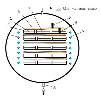
Figure: The diagram of vacuum drying plant with infrared transmitters VDSU-2M
