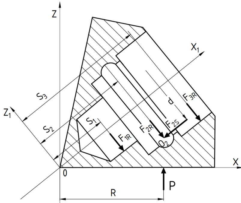
Fig 2: Scheme of forces acting on the rolling cone
