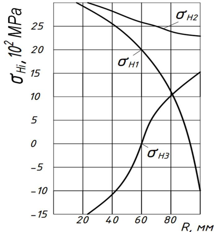
**Fig 5: Influence of the application radius of the external load on the calculated value of the maximum contact stresses in the support bearings**
