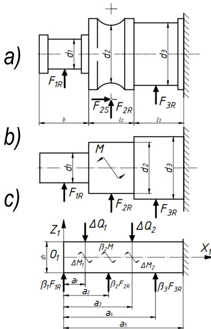
Fig 3: Scheme for calculating the deformation of the bearing pin
