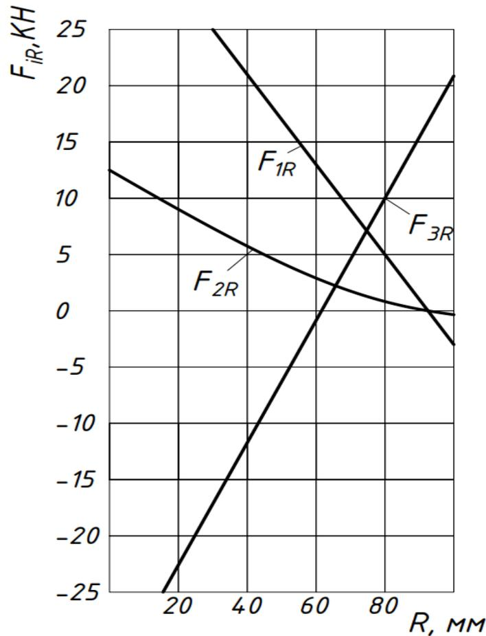
**Fig 4: Calculated dependencies of radial forces in bearings on the radius of application of external force (P=10 kN)**
