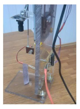
Figure 1: The scheme and the facility appearance; 1 – camera; 2 – the lights; 3 – crystal; 5 – table; 6 – incremental driver
