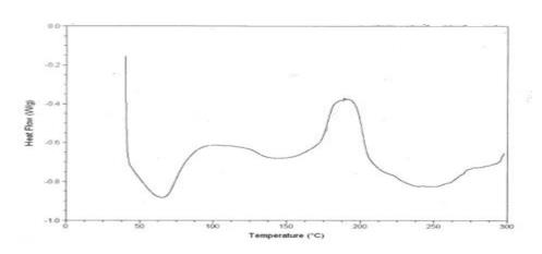
Fig 4: DSC thermo gram of AA copolymer -Ag Complex with more Ag concentration
