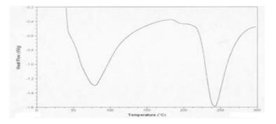
Fig 3: DSC thermogram AA copolymer -Ag complex with less Ag concentration.
