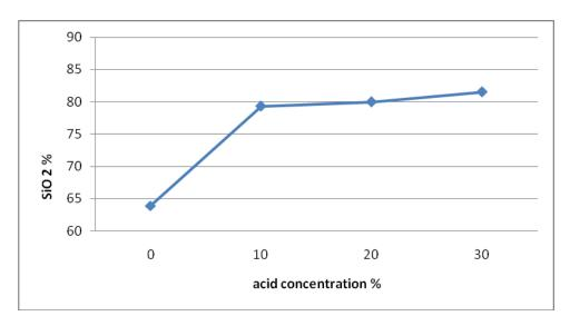
Figure 1: The relation between acid concentration and major component SiO<sub>2</sub> ratio
