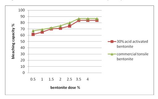
Figure 2: The relation between bentonte dose and bleaching capacity at 30% acid concentration
