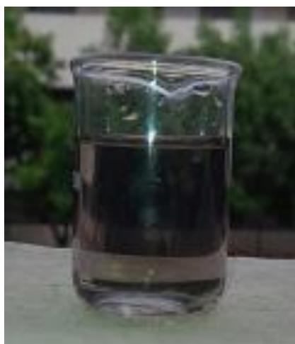
**Figure 3: Nanofluid prepared with 0.02% volume fraction of MWCNTs and distilled water as the base fluid**
