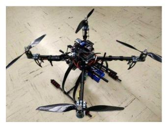
Figure 2. Assembled quadcopter test bed.
