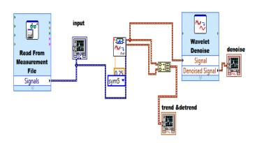
Fig. E. ECG signal Denoising
