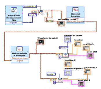
Fig. F. Peak detection block
