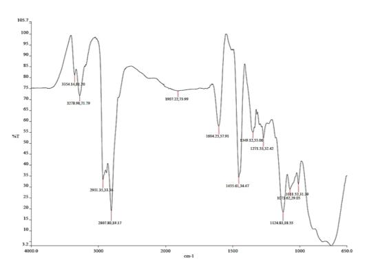
Fig. 4 IR spectrum of Waste PET with Triethylene tetramine - After 8 days
