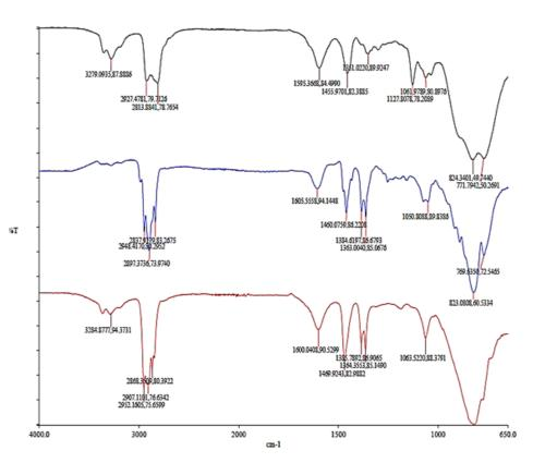
Figure. 8 IR spectrum of waste PET & Diethylene triamine blend , waste PET & Isophoron diamine blend & waste PET & Trimethyl hexamethylene diamine blend after 7 days
