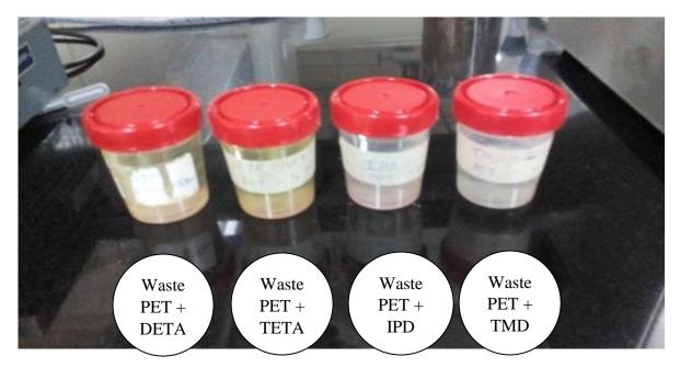
Fig.2 Dissolve the waste PET plastic pieces into Di ethylene triamine and Triethylene tetramine, Trimethyl, hexamethylene diamine, Isophoron diamine
