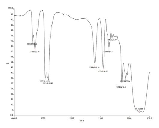
Fig. 5. IR spectrum of diethylene triamine
