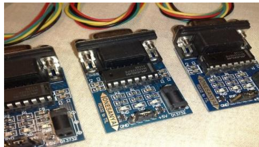
Fig. 12: RS-232 to TTL converters using MAX232
