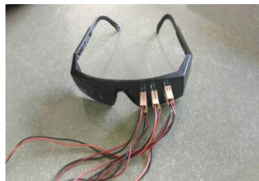
Fig. 4: Eye gear with three IR sensors
