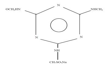
Figure 2: Scheme of poly melamine sulfone
