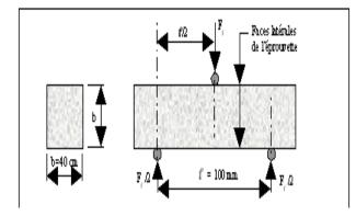
Figure 5: Device of bending load for the specimen's mortar
