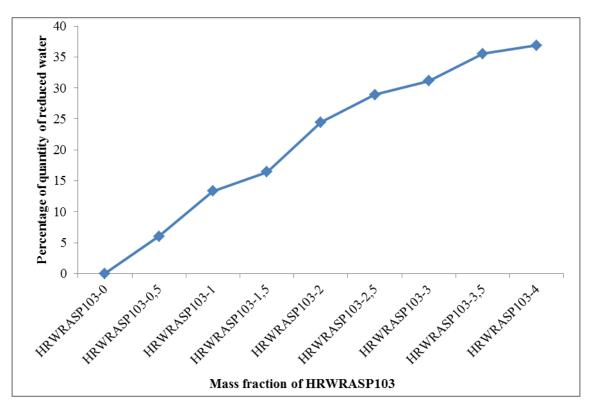
Figure 7: Variation of quantity of water reduced as a function of the mass fraction of HRWRASP103
