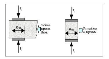
Figure 6: Device in compressive load for the specimens of mortars
