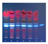
Figure 1: TLC chromatogram of extract from Soxhlet extraction using different solvent with different polarity: A) n-hexane, B) ethyl acetat, C) methanol, Soxhlet extraction with single solvent D) ethyl acetate, E) methanol, F). Extraction with maceration using methanol and S) sinensetin standard. Note: stationary phase silica gel GF<sub>254</sub> and mobile phase chloroform-athyl acetate (6:4)
