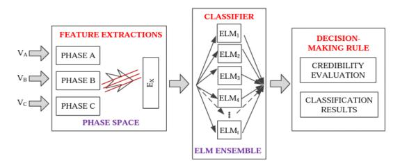
Fig.2: Structure of the phase space based ELM ensemble classifier
