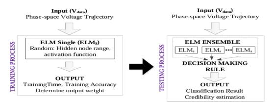
Fig.1: Description of inputs and outputs for the training and simulation data of an ELM-based ensemble classifier
