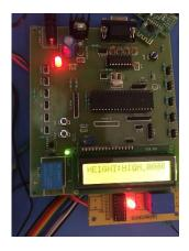
Figure 7.1: Reading of water level at the LED
