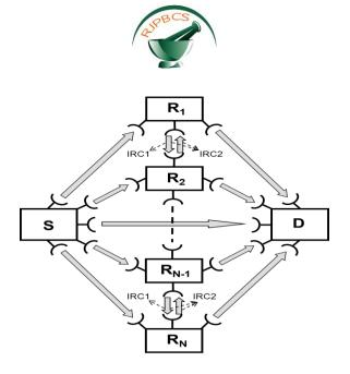
Fig 1: FSO relay-assisted transmission with N inter-connected relays
