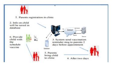
Figure 4: Architecture of the proposed system [4]
