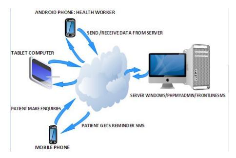
Figure 3: KenVACS system architectural design [2]
