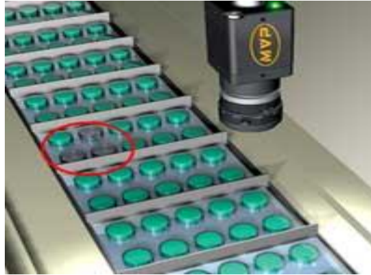
Fig.1: Inspection of tablets in industries
