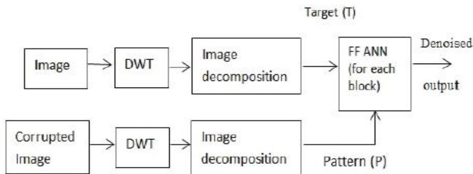
**Fig.1:the proposed method of multilevel-dwt based image de-noising using feed forward artificial neural network**
