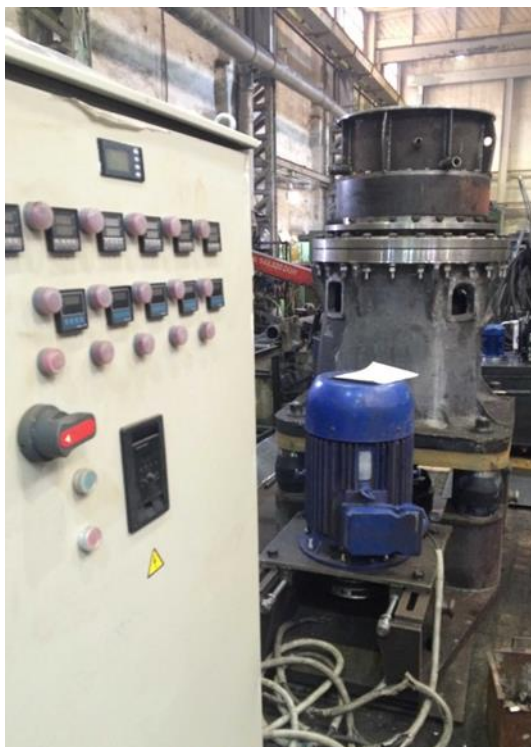
Figure 2 – Picture of a parabolic vibro-pulse grinder used for regrinding before brown coals heat treatment with the heat-treated coals further activation before separation. The equipment is undergoing the assembling and adjustment stage.
