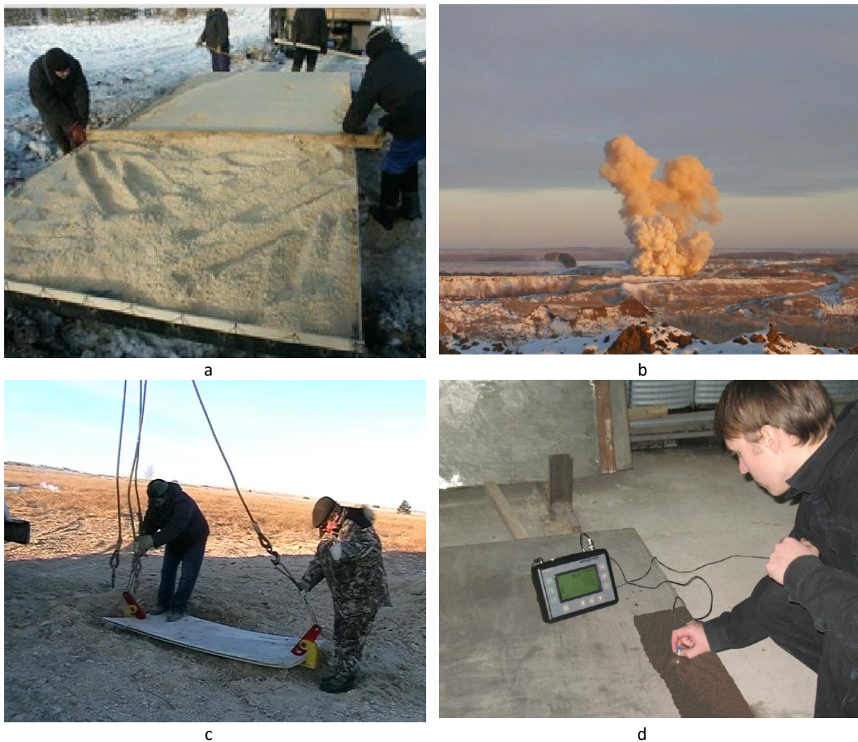
Figure 8. Working on the open testing ground and controlling multilayered materials: a – preparation for welding of a pile; b – blasting; c – loading the obtained metal block for transportation; d – ultrasonic control.
