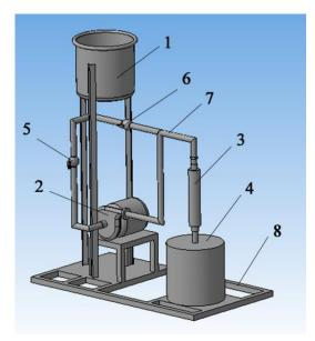
Fig. 1: Filtration installation design
