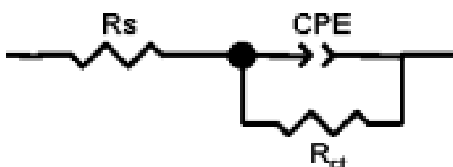
Figure 4. Equivalent electrical circuit corresponding to the corrosion process on the carbon steel in hydrochloric acid.
