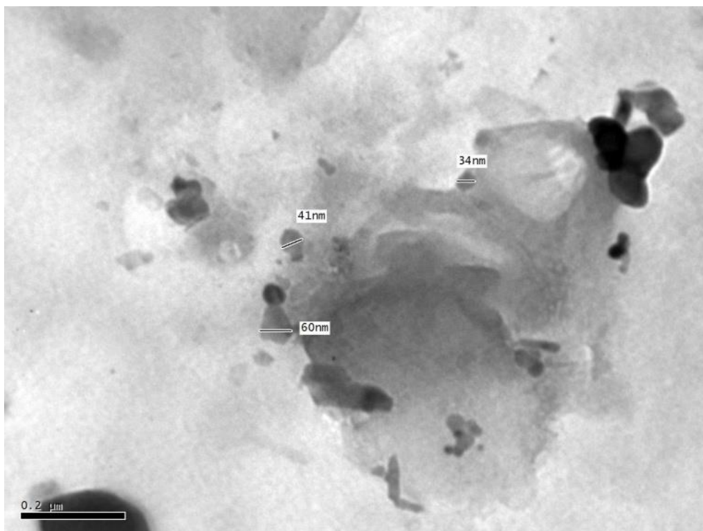
Fig 3: TEM of nano -silver prepared at \text{AgNO}_3 (1ml 0.1M) jatropa extract 4ml, 60°C, 150rpm, 15min and pH11.5.
