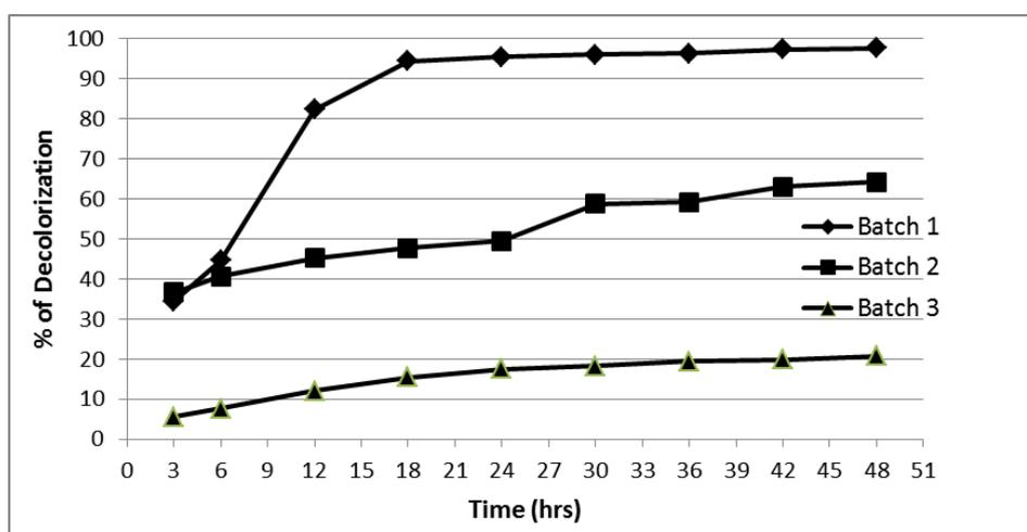
Figure 7. Basic Red 46 decolorization by *Enterobacter cloacae* sp. A3 in continuous fed batch process.
