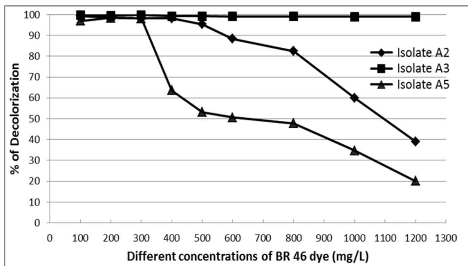
Figure 2. Effect of BR 46 dye concentration on decolorization performance of different isolates.
