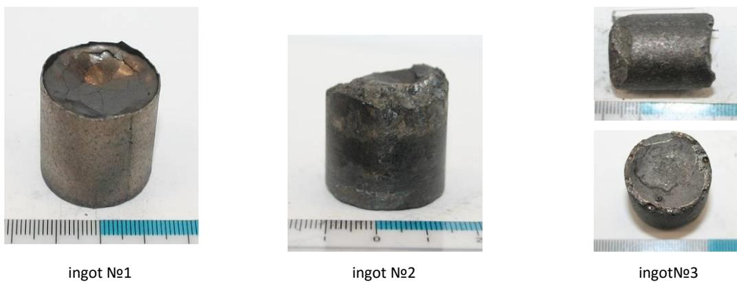
**Figure 2: Outward of corium ingots**
