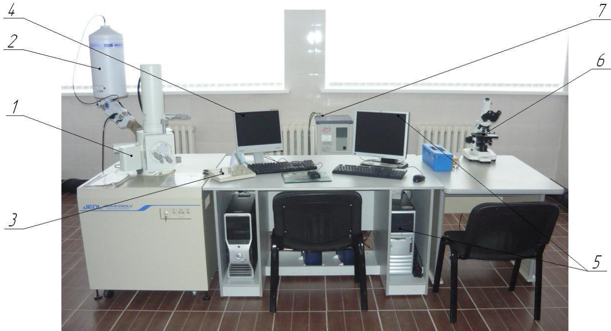
1 – Low vacuum analytical scanning electron microscope «JSM-6390LV JEOL»; 2 – system of X-ray microanalysis «INCA ENERGY 250, OXFORD INSTRUMENTS»; 3 – microscope control panel; 4 – computer for data processing of scanning observation; 5 – computer for data processing of X-ray microanalysis; 6 – binocular microscope “Mikmed-6”; 7 – water cooler.
