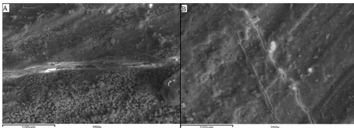
Figure (2): SEM micrographs showing the adaptation of the CSP after (A) one week immersion in deionized water at X 350. (B) one month immersion in deionized water at X 350
