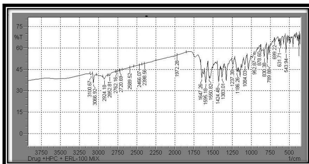
**Fig. 1: FT-IR of drug + HPC+ Eudragit RL-100 (physical mixture)**
