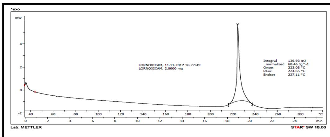
Fig.2: DSC thermogram of lornoxicam (pure drug)
