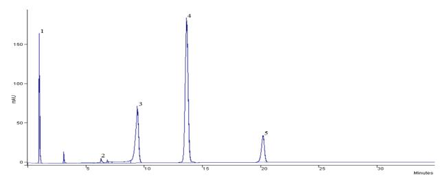
Fig 1: Chromatogram of reference standard mixture, fraction 1. Detection wavelength 320 нм. Peaks: 1 – ascorbic acid, 2 – caftaric acid, 3 – chlorogenic acid, 4 – caffeic acid, 5 – rutin.
