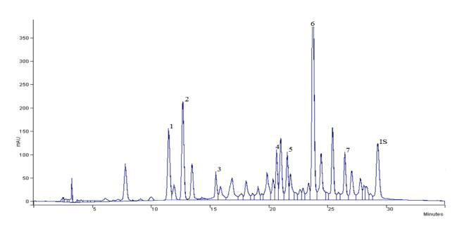
Fig 3: Chromatogram of Prostanorm liquid extract after SPE sample preparation. Detection wavelength 320 нм. Chromatographic conditions – gradient 1. Peak numbers correspond to substance numbers in table 1. IS – internal standard – salicylic acid
