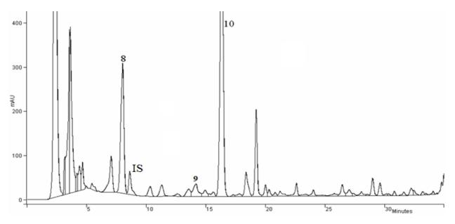
Fig 4: Chromatogram of Prostanorm liquid extract after SPE sample preparation. Detection wavelength 255 нм. Chromatographic conditions – gradient 2. Peak numbers correspond to substance numbers in table 1. IS – internal standard – salicylic acid
