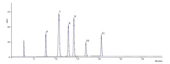
Fig 2: Chromatogram of reference standard mixture, fraction 2. Detection wavelength 320 нм. Peaks: 6 – hyperoside, 7 – chicoric acid, 8 – 2-hydroxycinnamic acid, 9 – quercetin, 10 – kempferol, 11 – glycyrrhizinic acid.
