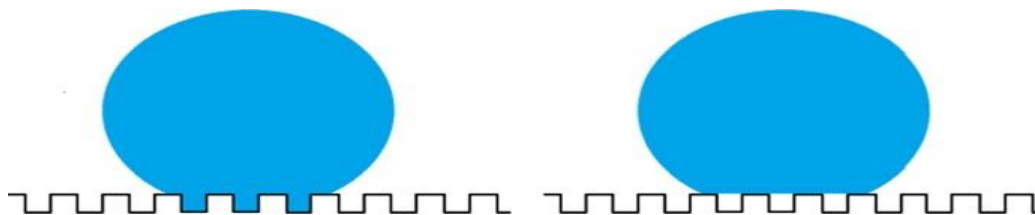
Fig. 2. (Top) Diagram showing the forces at the three-phase contact line of a liquid droplet on a solid; and (Bottom) Behavior of a liquid droplet on a rough surface: Left, Wenzel state and right, Cassie-Baxter state (Celia et al. 2013).
