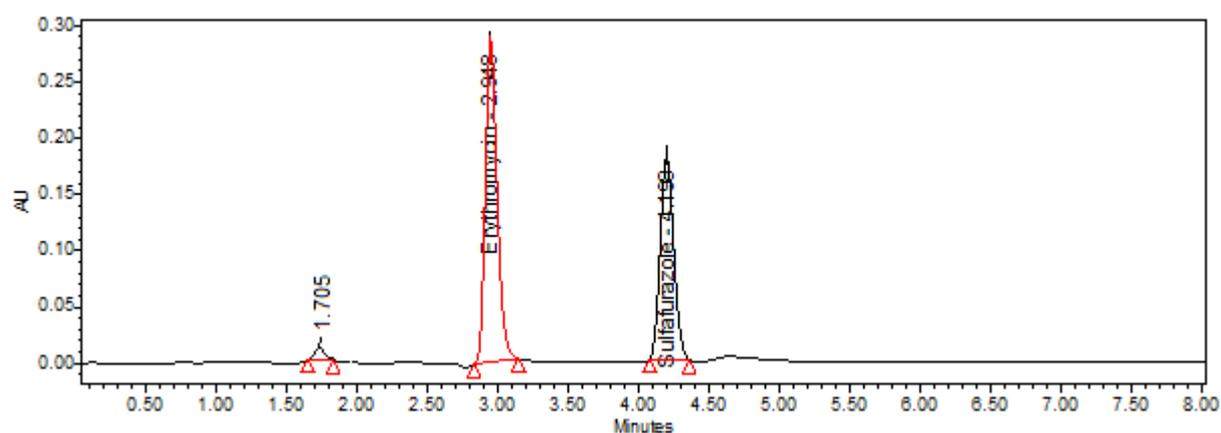
Figure 5: Chromatogram of erythromycin and sulfafurazole after photo degradation
