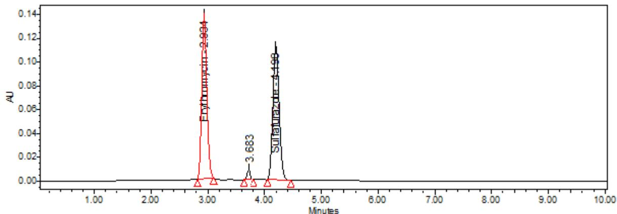
Figure 4: Chromatogram of erythromycin and sulfafurazole after oxidative degradation
