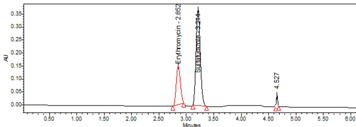
**Figure 3: Chromatogram of erythromycin and sulfafurazole after alkali degradation**
