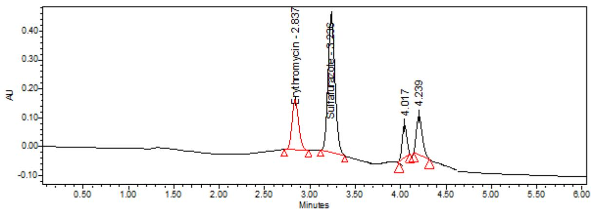
**Figure 2: Chromatogram of erythromycin and sulfafurazole after acid degradation**
