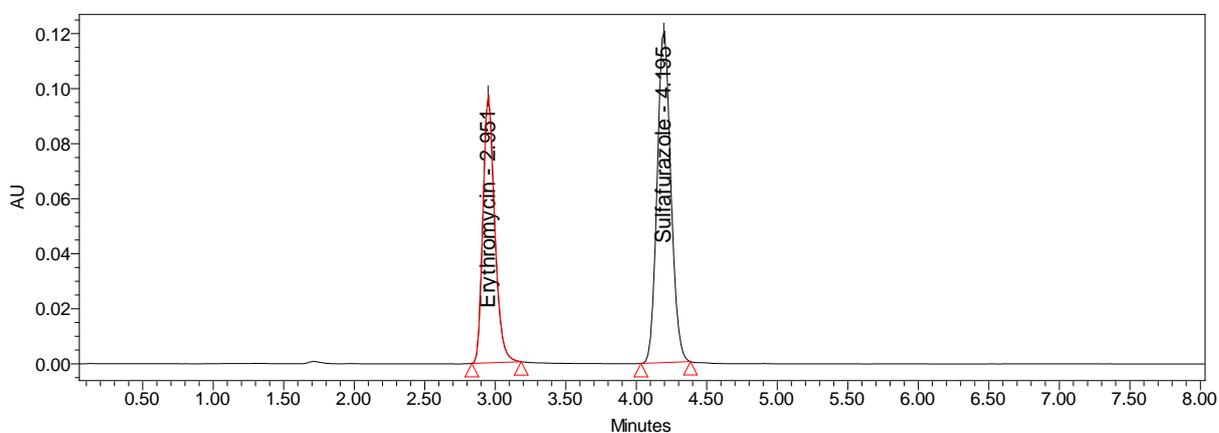
**Figure 1: Chromatogram of erythromycin and sulfafurazole under optimized conditions**
