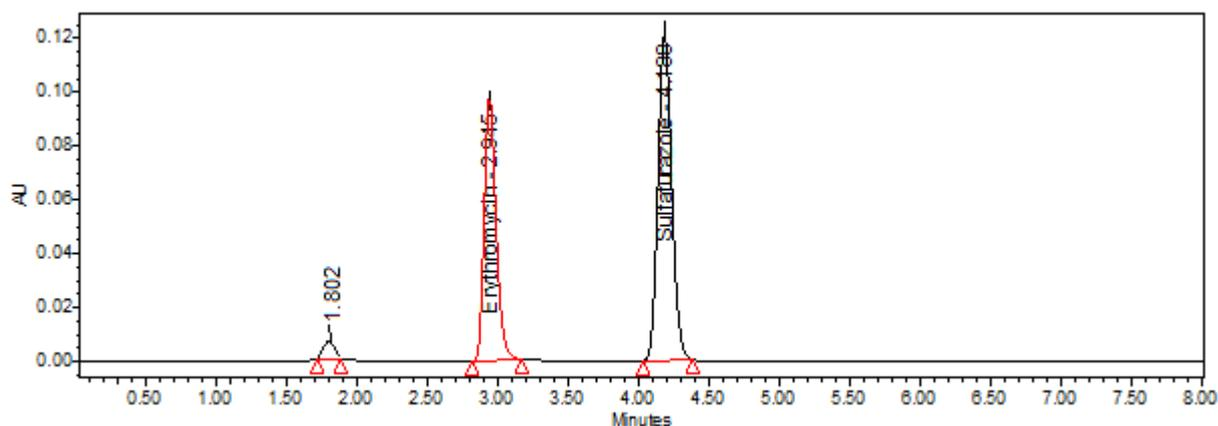
Figure 6: Chromatogram of erythromycin and sulfafurazole after thermal degradation
