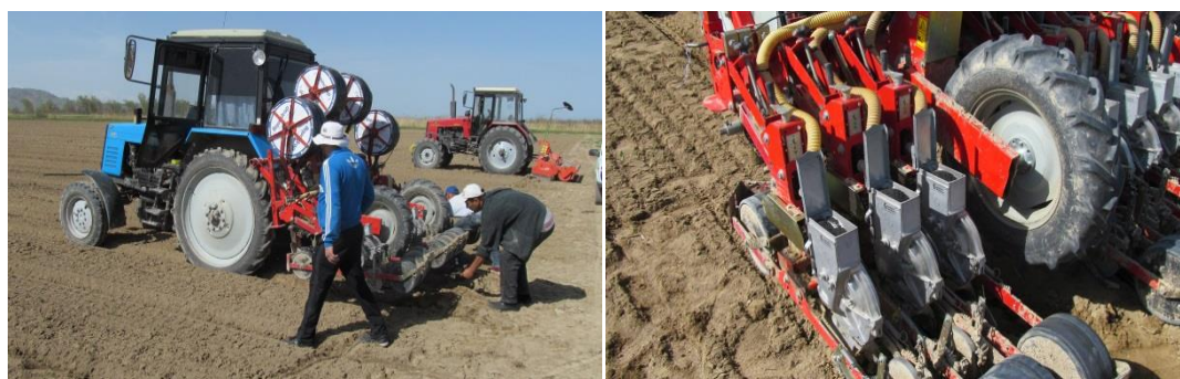
Figure 4. Onions planting with simultaneous laying of lines for subsurface and drip irrigation
