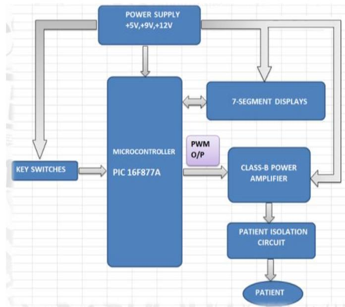
Figure 1. Block Diagram
