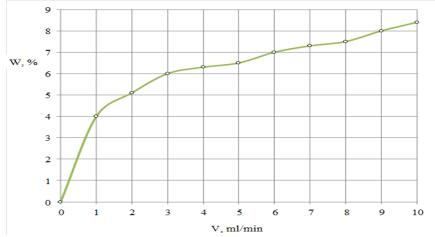
Picture 2 – Change of moisture mass fraction in the product depending on the solution feeding rate in a solution with lactulose mass fraction of 50 %
