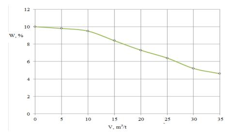
Picture 1 – Change of moisture mass fraction in the product depending on the airspeed in a solution with lactulose mass fraction of 50 %
