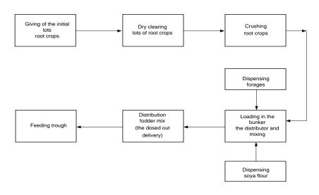
Figure 2: Block diagram of the process of preparation and distribution of feed mixtures for pigs
