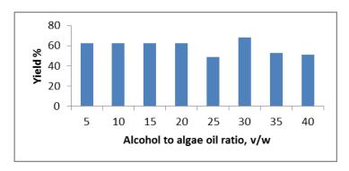
Figure 4: The effect of alcohol to biomass oil ratio the yield % of FAME
