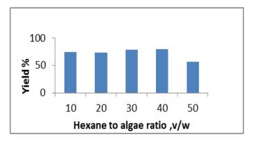
Figure 2: The effect of co-solvent ratio on the yield % of FAME
