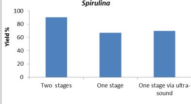
Figure 5: Comparison between different methods of transesterification
