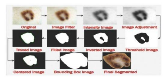
Figure 7: Schematic representation for image Segmentation steps
