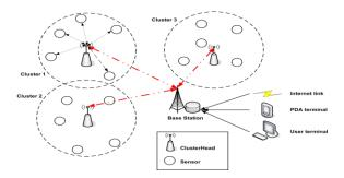
Fig: 1 Block Diagram of WSN
