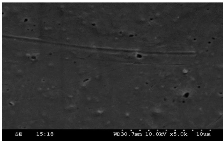
**Figure 4: SEM of the film formed upto 220V in 0.1M L-ascorbic acid (glycolic medium) at room temperature (Magnification of the micrograph is X 5000)**
