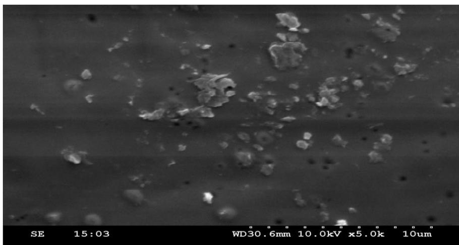
Figure 3: SEM of the film formed up to 220V in 0.1M L-ascorbic acid (aqueous medium) at room temperature (Magnification of the micrograph is X 5000)
